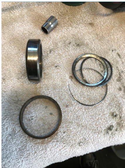
Bearing and shims. Notice the thin shim caused by rotation against the bearing edge.
