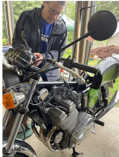
Paul demonstrated how to balance the carburetors on his three cylinder Laverda 1200
