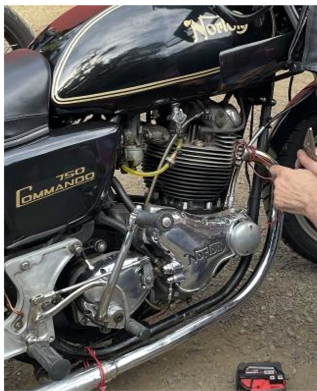
Red hookup wire holding the pipe. No rocks necessary for this repair!
